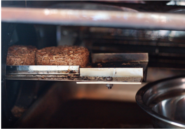
Briquette feed mechanism on a Bradley digital smoker.
