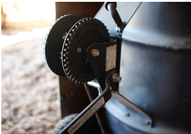
Winch for raising or lowering grates in the drum of a homemade charcoal smoker.
